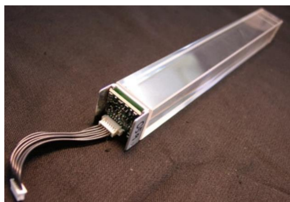
Detection channel. PWO crystal glued with photodetectors. APD and SiPM mounted on the preamplifier's substrate. The CSP and the current preamp on a printed circuit board of area 19 mm x 19 mm are mounted to the back side of the photodetectors.
